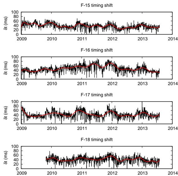
**Figure 3.** Timing shift time series (black) for DMSP satellites from January 2009 through July 2013, except for F-18 which was launched in October 2009. Red curves show smoothing splines used for final timing signal.
