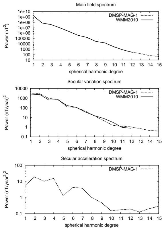
**Figure 10.** Main field, secular variation and secular acceleration coefficients of DMSP-MAG-1 compared with WMM2010 (WMM2010 does not provide secular acceleration).
