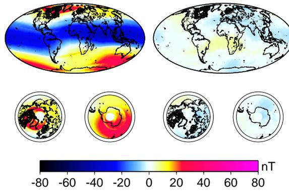
**Figure 6.** Pomme-8 scalar residuals for F-16 averaged over 2010 gridded in latitude and longitude prior to calibration (left) and after calibration (right).
