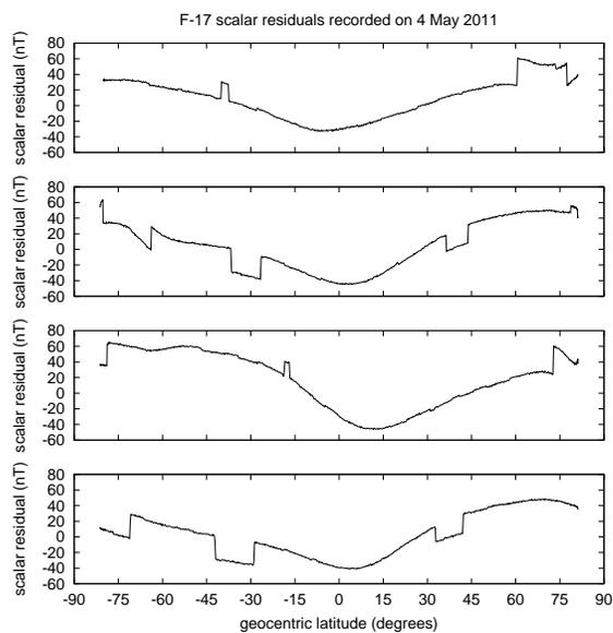
**Figure 1.** Samples of DMSP scalar residuals after subtracting Pomme main field model for several orbital tracks. Data were recorded by F-17 on 4 May 2011.
